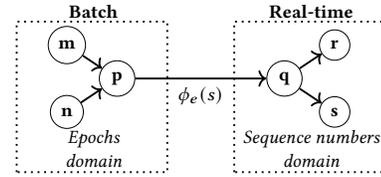
**Figure 3: Application composed of a batch and a real-time component. The components have different fault tolerance requirements, and thus use different logical time domains.  $\phi$  bridges between the domains.**
