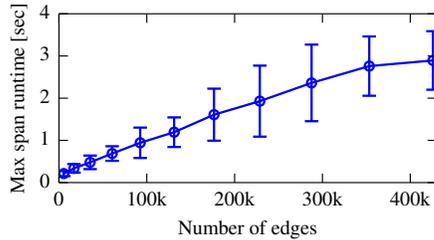
**Figure 10: Span monitor scalability. The slowest component of the monitor, the algorithm for choosing maximal spans for rollback, scales linearly with the number of edges.**
