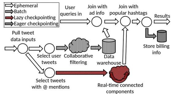
**Figure 1: An example ad-serving application comprised of several batch, streaming, and iterative components. Each component uses a different fault-tolerance regime.**
