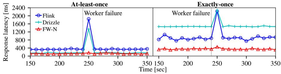
**Figure 8: Latency during failure recovery. FW-N has up to 10× lower mean response latency during failure recovery, both with at-least-once and exactly-once semantics. Results on YSB executed on 25 machines.**
