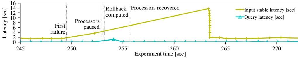
**Figure 5: Latency of different application components during failure recovery.** FW-N allows query latency to remain low despite three machine failures (at around 250 seconds), masking the longer recovery time required for the latency of batch input processing to return to its normal levels.
